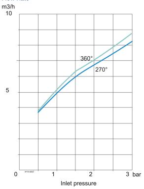
For Clip-on models, the flow rate is increased by approx. 0.5  $\mbox{m}^{3}/\mbox{h}.$
